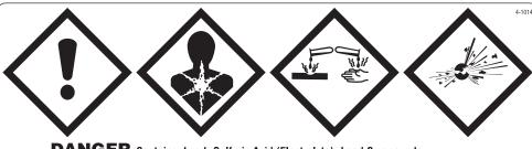
**DANGER** Contains: Lead, Sulfuric Acid (Electrolyte), Lead Compounds.
