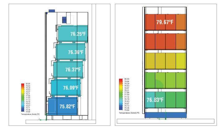
It is vital to remember that standard lead acid battery design life and ratings is most favorable at 77°F (25°C).
