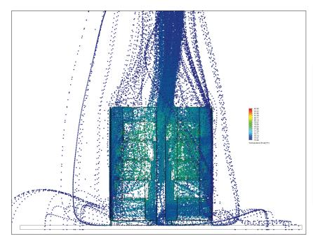
These images depict complete modeling of C&C Power UBC "CoolCab" with forced air cooling and Deka front access batteries.
