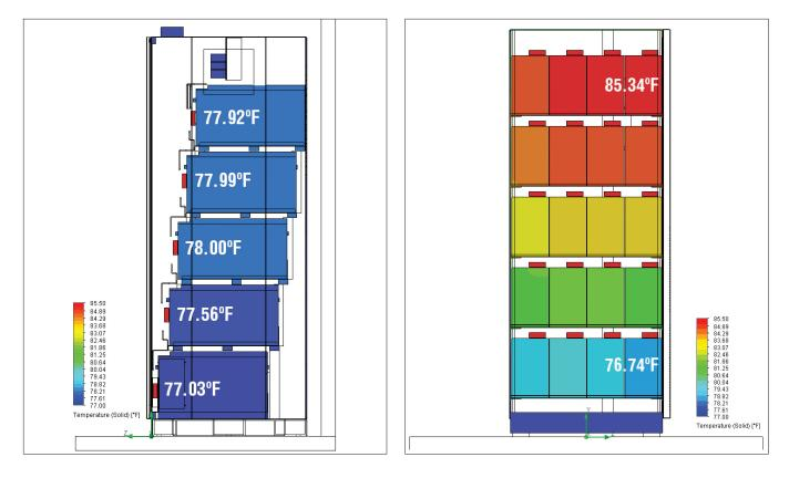
The airflow directly impacts the batteries temperature above ambient, stratification of battery temperatures within the battery cabinet, and overall battery life.
