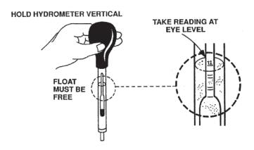
The correct hydrometer reading corresponds to an imaginary line drawn across the side of the barrel at the lowest level of the electrolyte. If the hydrometer has to be removed from the vent hole, pinch the nozzle tightly or place a gloved finger against the opening to prevent dripping.
