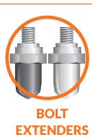
DO NOT USE Battery Bolt Extenders or Battery Bolts for testing or charging batteries. They do not provide the necessary lead-to-lead contact, and can reduce your cold cranking amperage (CCA) and state of charge readings. Batteries should be boost charged if the open circuit voltage (voltmeter) reading is below 12.4 volts. See charging chart below.
