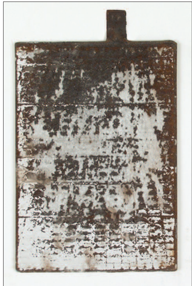
A plate formed in the battery case. White areas indicate plate is not fully formed.
