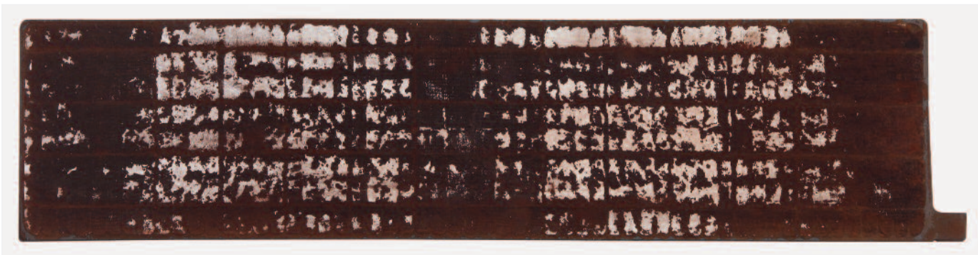
Competitor's plate formed in the battery case. White areas indicate plate is not fully formed.
