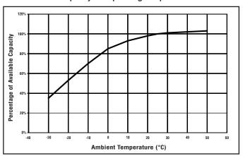
Capacity vs. Operating Temperatures: Above are the changes in capacity for wider ambient temperature range, giving the available capacity, as a percentage of the rated capacity, at different ambient temperatures. The curves show the behavior of the battery after a number of cycles.
