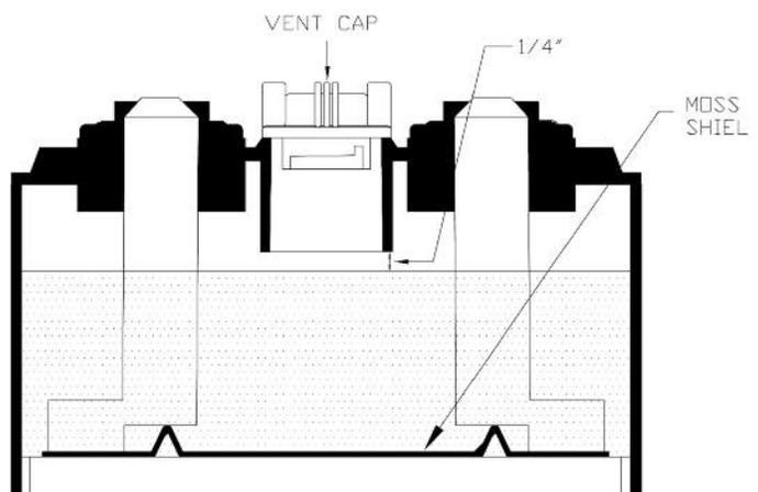
If a large amount of liquid is required to raise the level, the battery may be damaged. Inspect the packing material under the tray for signs of leakage. All damaged components should be inspected by your East Penn agent or representative.
