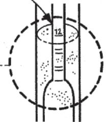
The correct hydrometer reading corresponds to an imaginary line drawn across the side of the barrel at the lowest level of the electrolyte. If the hydrometer has to be removed from the vent hole, pinch the nozzle tightly or place a gloved finger against the opening to prevent dripping.
