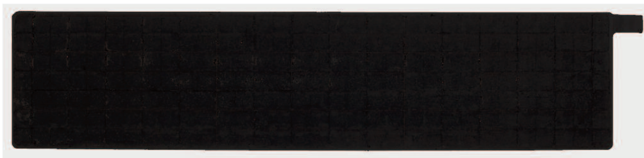
Fully formed Deka plate using East Penn’s formation processes.
