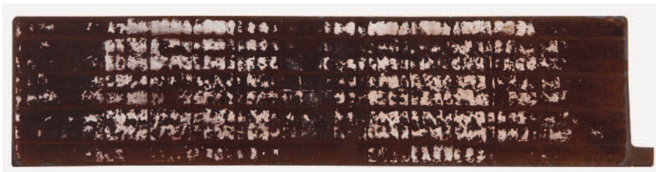
Competitor’s plates. White areas indicate plate is not fully formed.
